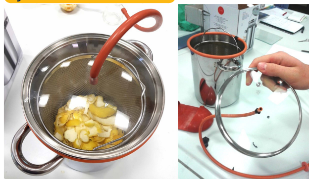
Fig. 2 Steam distillation of lemon zest
