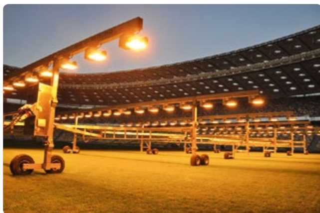
FIG. 1 Lighting rigs to speed up grass growth
