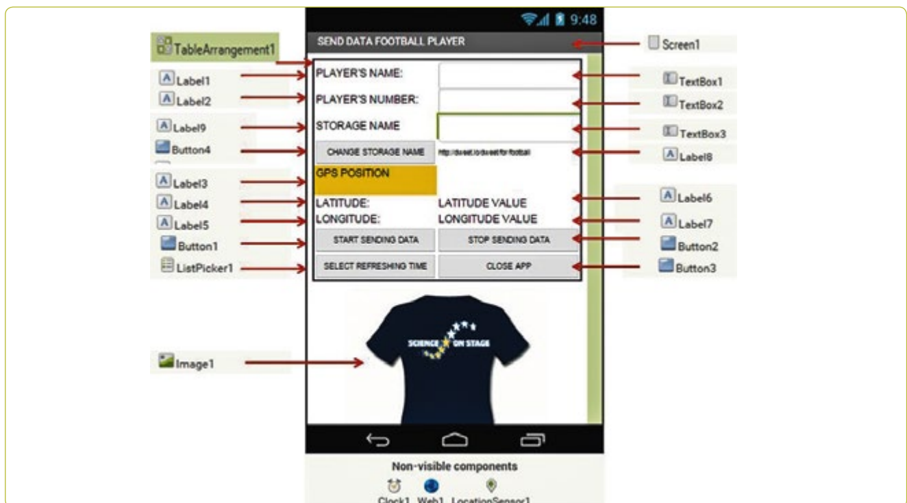
FIG. 2 Components of TableArrangement1
