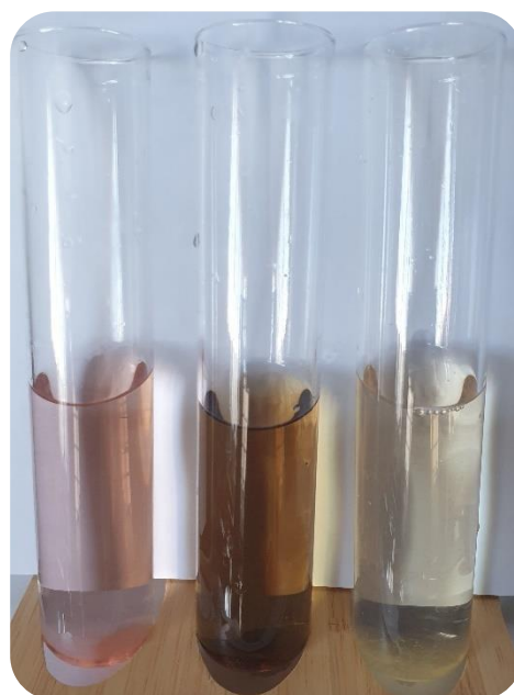
Figure1: Tube 1: hibiscus tea; Tube 2: hibiscus tea with sodium percarbonate; Tube 3: hibiscus tea with sodium dithionite
