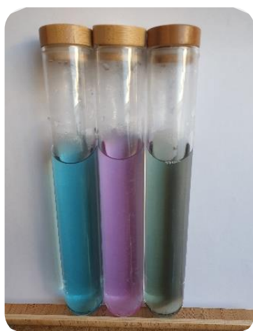
Figure1: Infusion of butterfly pea flower tea (left); after adding lemon juice (centre); and after adding ammonia (right).
