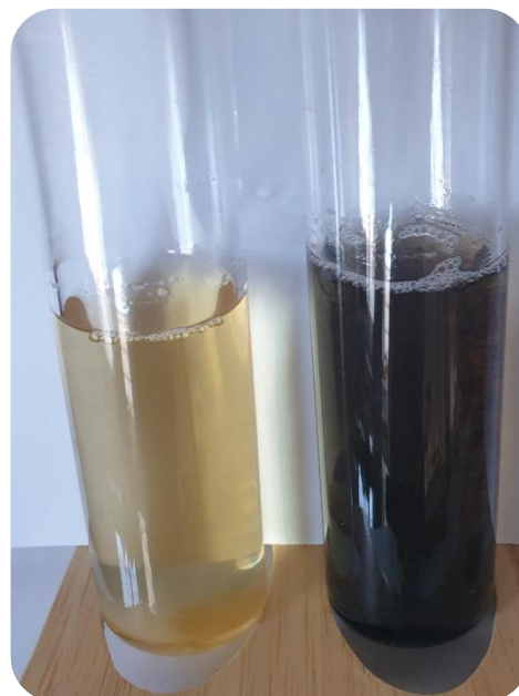
Figure 1: An infusion of black tea (left), and after adding an aqueous solution of iron(III) chloride (right)
